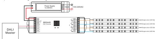
2)Connection Diagram for Multiple Units
